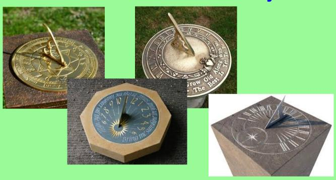
As the earth turns, the sun appears to move across the sky. This apparent motion gives us day and night. A sundial uses the position of the sun in the sky to tell the time. The time measured by a sundial is solar time...
